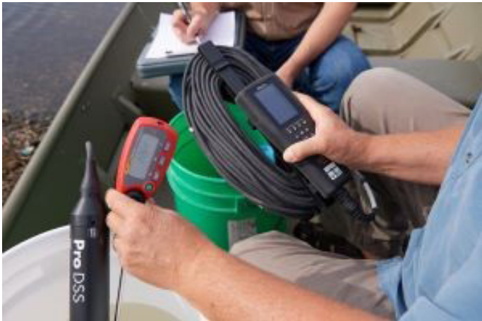
Mark uses a 1551A-EX Stik Thermometer to calibrate the multi-probe
